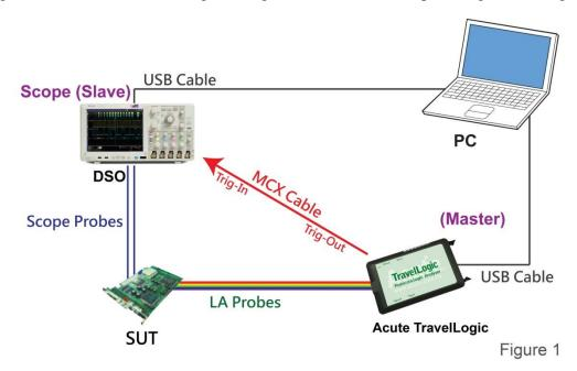
In Figure 1, the USB or Ethernet (TCP / IP) interface is connected to the computer, and then connect the BNC-MCX cable to the TravelLogic Trig-Out and the trigger input interface (Ext-Trig, Aux In or Trig-In) of the oscilloscope. MDO4000 series is fixed in the analog channel CH4.
