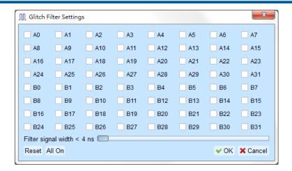
This filter function can be set to filter the signals of less than 5ns-35ns wide. After this filter function is enabled, it will filter before the hardware is triggered. Channels that use the glitch filter function are marked with a red dot on the channel label for identification.
