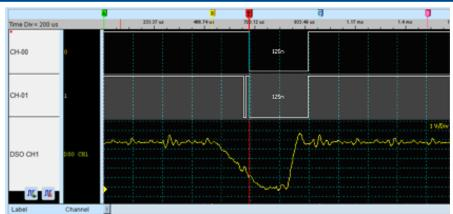
The use of a hardware surge filter (that is, Low-Pass Filter) may filter out the noise (Glitch) and solve this problem, but may filter out true noise or high frequency signals. Therefore, the use of hardware surge filter is not suitable for solving such problems.
