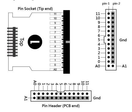
26-pin eMMC connector: Probe tip = Pin socket, Pitch=2.54, Unit: mm.
