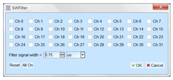
This filter function can be set to filter the signals with pulse width range from 1ps to 1ms. Applying this filter function will only change the display and decode contents, the trigger and recordable time will remain not effected. Disabling this filter function will restore all waveform contents back to the original un-filtered waveform.
