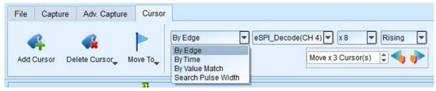
1. By Edge: Move the specified cursor position according to the number of Rising / Falling / Either edges ( $x1 \sim x4096$ ) of the specified channel.
