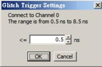
ONLY Channel 0 (default) can be the glitch trigger channel. Parameter range:  $0.5 \sim 8.25$
