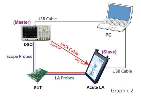
Connect the DSO (Trig-Out) with the logic analyzer (Trig-In) over a MCX-BNC cable for the Tektronix/Agilent/GW Instek DSO (MCX-MCX cable for Acute DSO); connect the DSO with the PC over an USB or Ethernet cable.
