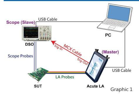
Connect the logic analyzer (Trig-Out) with the DSO (Trig-In or Ch4 for Tektronix MDO4000 serial) over a MCX-BNC able for the Tektronix/Agilent/GW Instek DSO (MCX-MCX cable for Acute DSO); connect the DSO with the PC over an USB or Ethernet cable.
