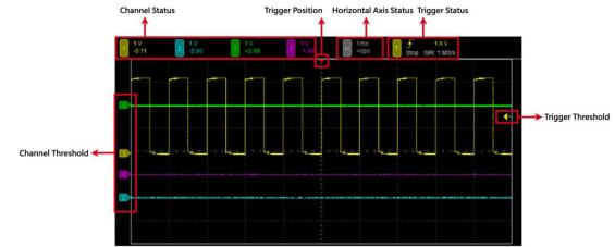
Channel StatusShows the VOLT/DIV and the status of different channels.Single click on the channel icon to enter the channelsettings dialog. Please refer to <a href="https://channel.settings">Channel Settings</a>.
