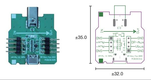
Processing the DP\_Aux signal into a single-ended signal for measurement.
