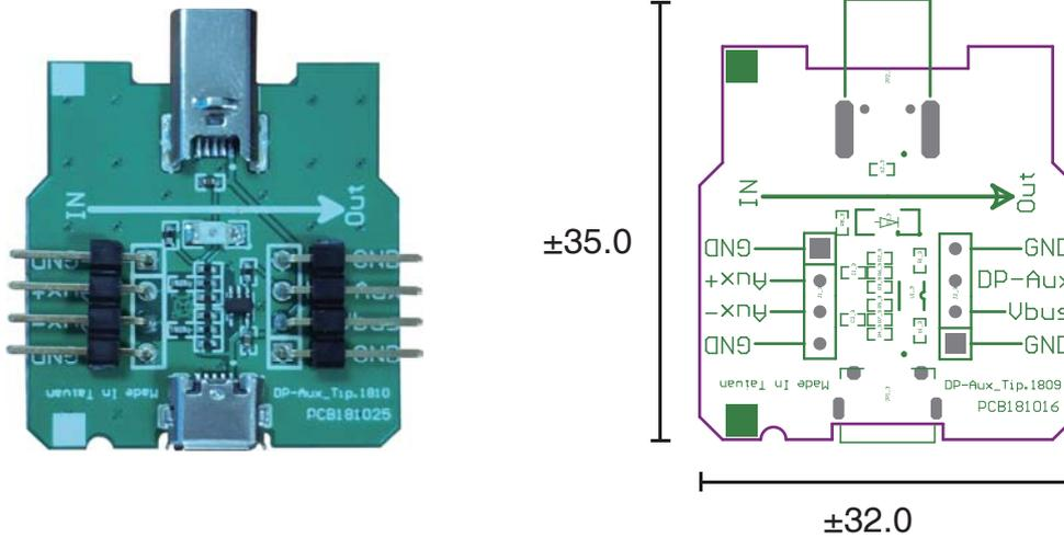
Processing the DP\_Aux signal into a single-ended signal for measurement.
