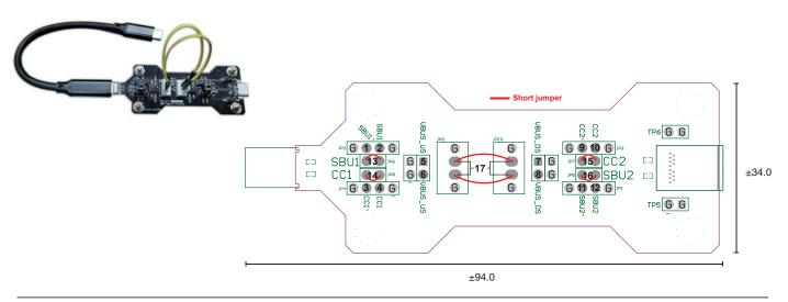
This fixture the PD signals CC1, CC2, and DP\_Aux, as well as the SBU1 and SBU2 signals from the Type-C connector, enabling convenient testing with a logic analyzer without damaging the Type-C Fixture.
