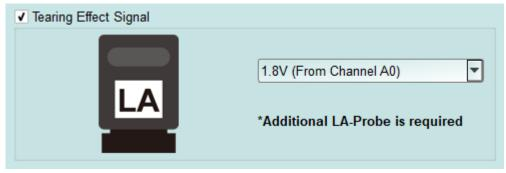
Detect the TE signal from the screen. Must purchase LA Probe to use this function.
