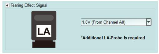
Detect the TE signal from the screen. Must purchase LA Probe to use this function.
