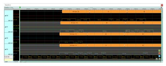
Ex: The width of high pulse in Lane 0, Lane 3 is not the width of half CLK cycle Half CLK cycle = (1.4 + 0.8) / 2 = 1.1 (ns)
