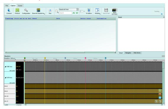
Since the analysis of NAND Flash requires the use of more channels, an LA probe needs to be connected to Slot A, and it can only be turned on using a sampling rate of 1GHz.
