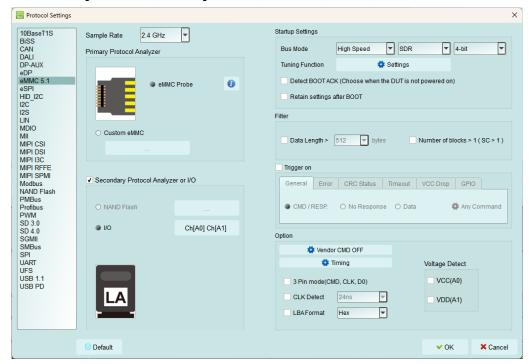
While using the eMMC 5.1 protocol analyzer, you can additionally enable the NAND Flash logic analyzer function or additional I/O pins for analysis.
